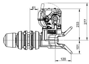
4: The distance to the coupling centre "L3" varies depending on the compression of the rubber element as well as the drawbeam thickness (see table).
